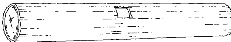
Figure 8 Barking a Patch for Bark Thickness Measurement
